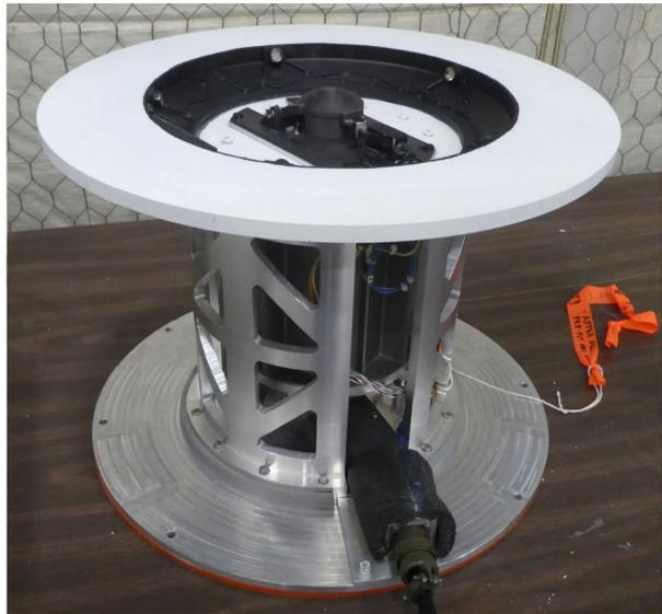
Sumner, New Mexico. The unique ASHI design includes a corral (the white cylindrical disk at the top of the instrument). This has a 2° curved surface that reduces the light shining from below it onto the fisheye lens in the center of the corral by more than 10 orders of magnitude
