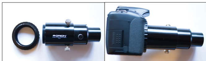
Fig. 2. Eyepiece projection setup. On the left the eyepiece projection adapter and a T-ring are shown. On the right the completed connection is shown (the eyepiece is inside the adapter and cannot be seen).
